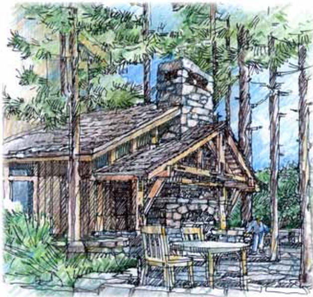
Figure 3.7: Stone foundation wall transitions to a chimney, anchoring building to site.
